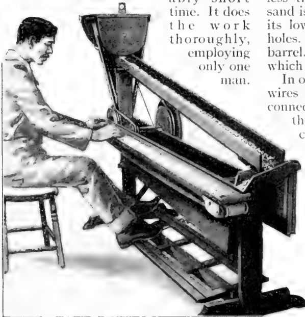
One workman using the machine can clean and sort a large quantity of beans in a remarkably short time
